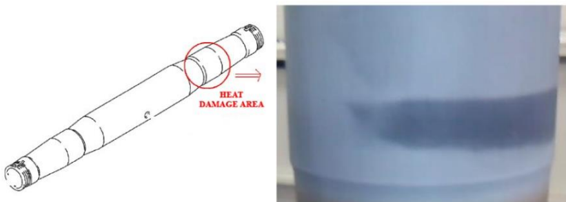
Figure 4. B737-800 MLG inner cylinder strut area where thermal damage occurs
