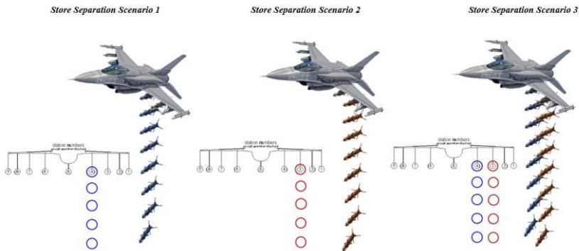
Figure 3. Scenarios of Store Separation from Different Pylons.
