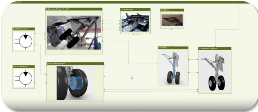
Figure 22: Landing Gear Subsystem Logical Architecture (Source: Dassault Systems, 2021 (3DEXperience PLM 2021x))
