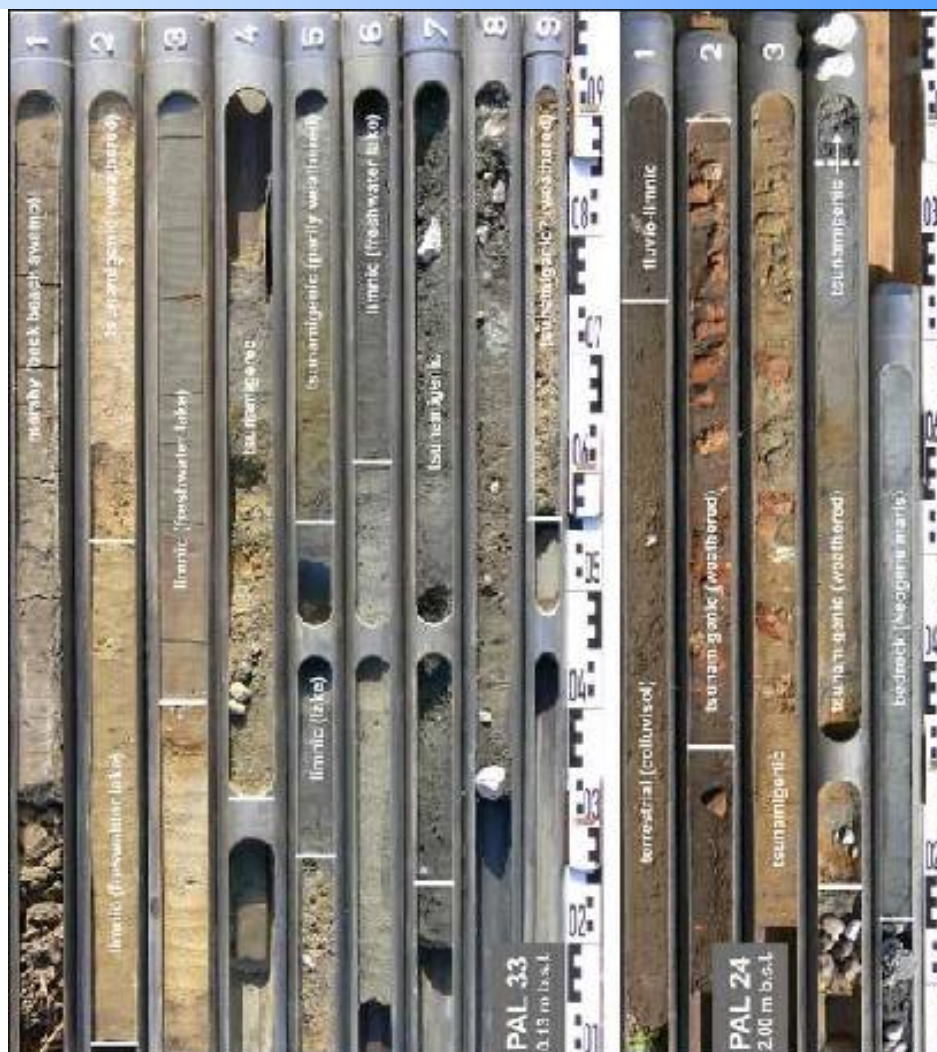
Figure 25. (a) A 9-m core with at least five tsunamigenic layers (often with grading up) from Palairos, NW coast of Greece. (Image credit: Vött et al., 2011c).
