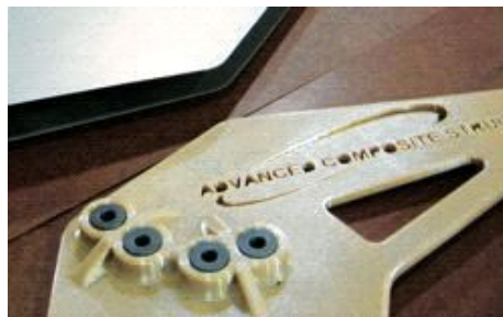
Figure 8. Hole drilling fixture manufactured by Advanced Composite Structures company by FFF (Anon n.d.)
